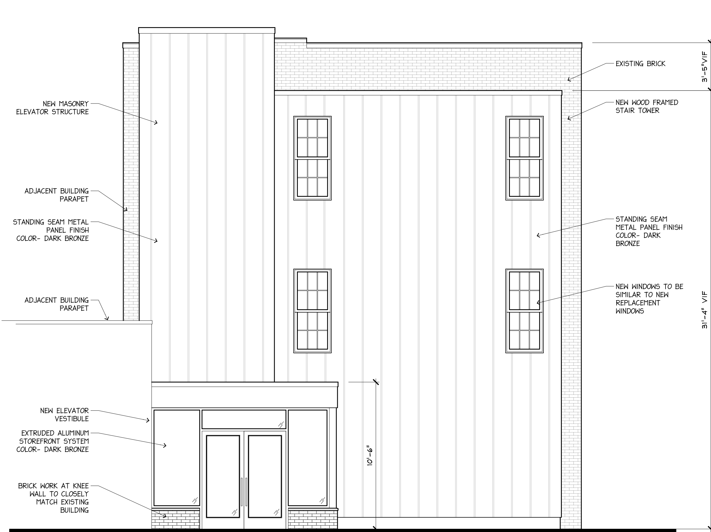
2 WEST ELEVATION - REAR SK1 1/4" = 1'-0"
