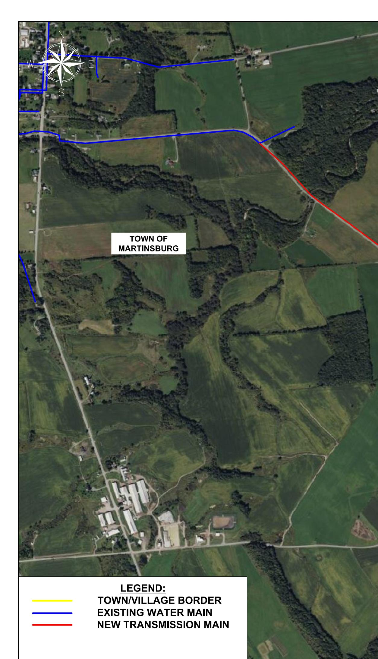
**NEW 8-INCH DUCTILE IRON TRANSMISSION LINE**
